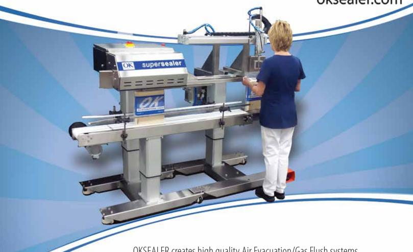
OKSEALER creates high quality Air Evacuation/Gas Flush systems. Air Evacuated/Gas Flushed, sealed bags, extend the shelf life, and/or reduce volume for packaging.
