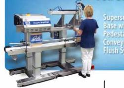
Supersealer SB20 (Right to Left) Base with Casters & Motorized Pedestal with Optional BBY-100 Conveyor and Air Evacuation/Gas Flush System.
