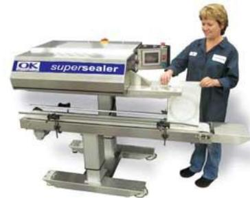
Of all available technologies, band sealers can handle the widest variety of bag materials, from paper, poly, and foil to Tyvek®. They're the recommended sealing solution for Tyvek® pouches and Tyvek®/Mylar® pouches. Because of the hills and valleys in Tyvek®, the physical contact the band provides is essential. The bands hold the film, so heat can't cause wrinkling or shrinkage during the sealing process.
