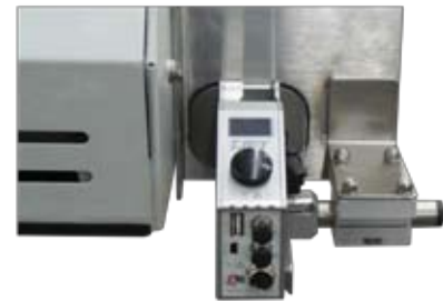
iJet Thermal Ink Coder mounted at exit of Supersealer SB10
