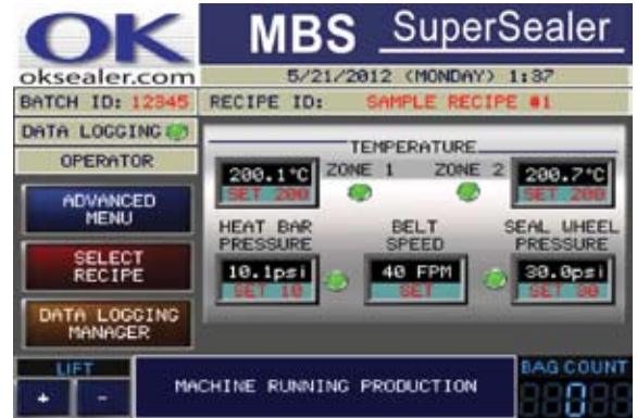
Touch screen operator interface for easy system and control monitoring
